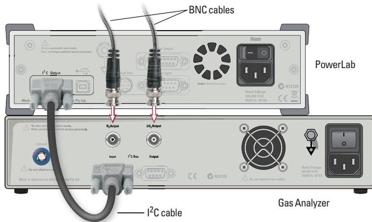
Use two BNC cables to connect the CO<sub>2</sub> and O<sub>2</sub> analog outputs on the back panel (Figure 2-1) of the Gas Analyzer to two available inputs on the front panel of your PowerLab. Any free inputs on the PowerLab can be used for other measurements.
